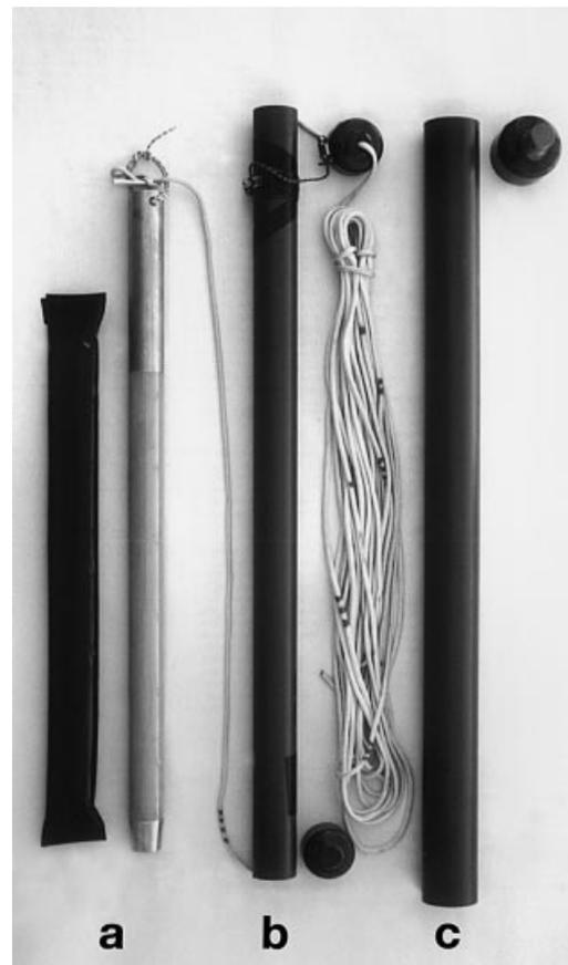
Fig. 2. Photograph of the experimental set up for obtaining sulphur prints from the sediment. (a) Stainless steel tube (4 cm diameter) with PVC foil cover; (b) outer PVC tube with lids to avoid exposure to light; (c) PVC tube for fixation process of the photographic paper. The lengths of the PVC tubes are  $\approx 1 \text{ m}$ .
